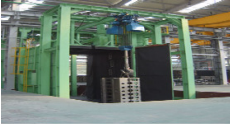
Shot Blast Machine: • 1×20MT/batch1
