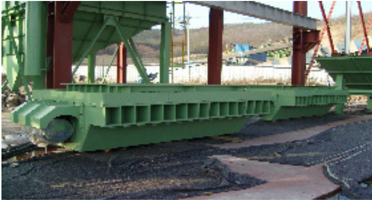
Shake out machine: • 1×20MT/hour
