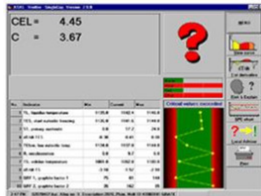
Artificial intelligence technology judges the quality of tested melt
